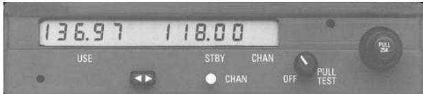
b. GA aircraft VHF radio equipment typically has 760 channels spaced at 25 kHz; some older radios may have only 720 channels with an upper limit of 135.975 MHz, these are not allowed for IFR flight, or for VFR flight in certain countries including Germany.
